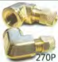
270 FEMALE ELBOW FITTING Female Pipe to Compression 90° Elbow For Nylon and Polyethylene Tubing. Brass.
