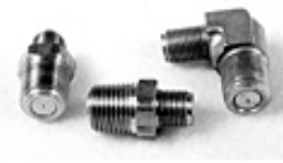
4022 & 4023 PRIMER FITTING Has .040 Internal Orifice. 1/8-27 NPT 5/16-32 Thread. Straight or 90° Elbow.
