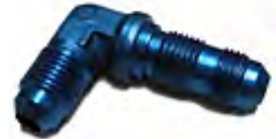
AN833 ELBOW FITTING Bulkhead 90° Flared Fitting
