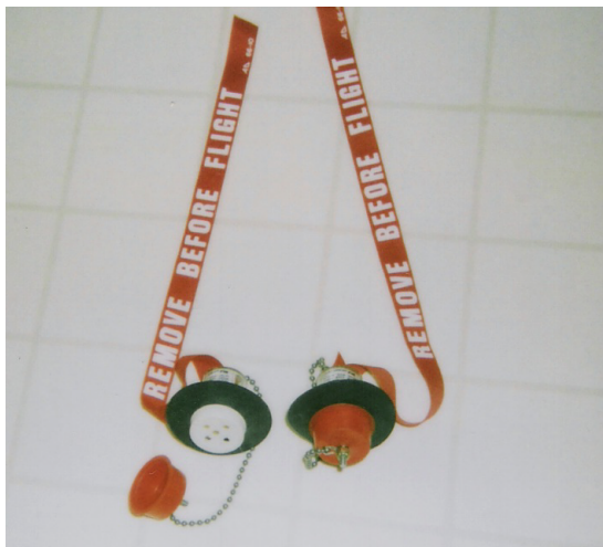
PICTURE SHOWING THE ENGINE DEHUMIDIFER INSERTED INTO THE EXHAUST PIPE KEEPING THE ENGINE AIR DRYER THAN IT WOULD NORMALY BE
