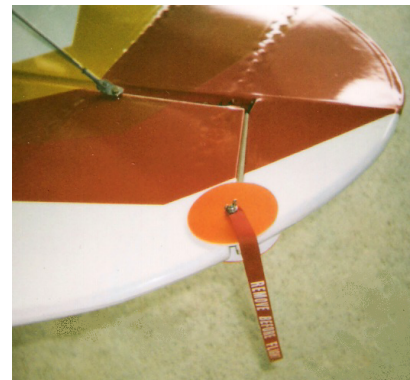
TYPICAL ELEVATOR LOCKED
