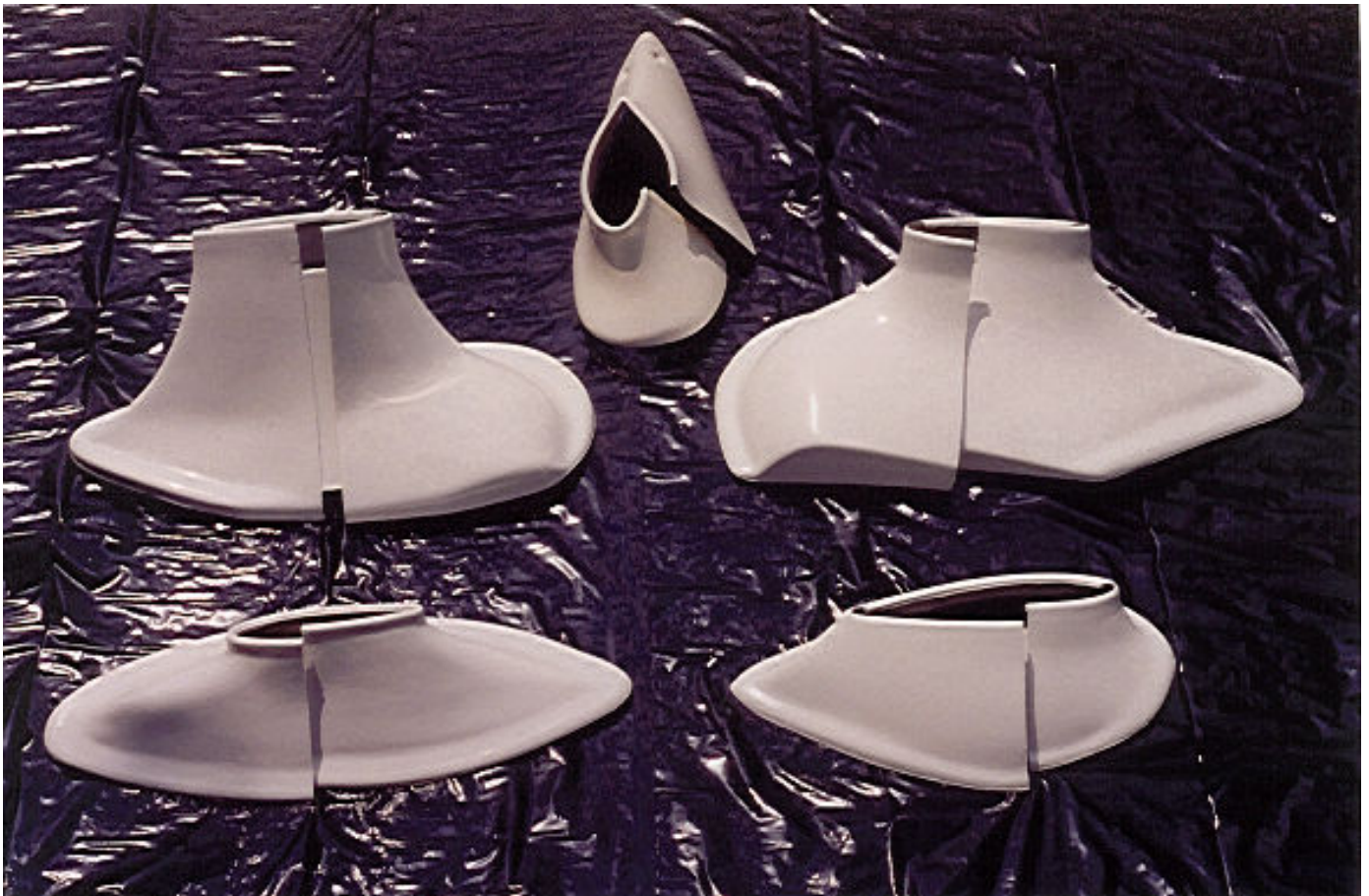
PICTURE SHOWING SEVERAL TYPICAL CESSNA LANDING GEAR STRUT FAIRINGS
